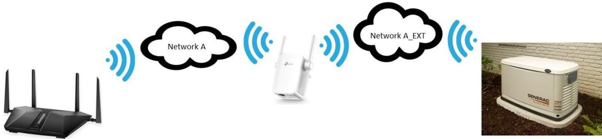
**Note** – If you have a TP-Link network extender installed between your wireless router and the generator and the router password, router, or wireless name changes, you will need to re-attach the network extender to the wireless network
