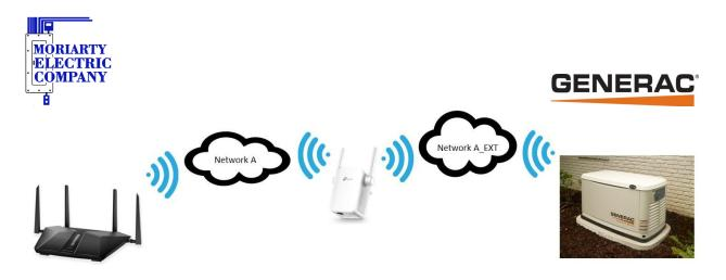
**Note** – If you have a TP-Link network extender installed between your wireless router and the generator and the router password, router, or wireless name changes, you will need to reattach the network extender to the wireless network
